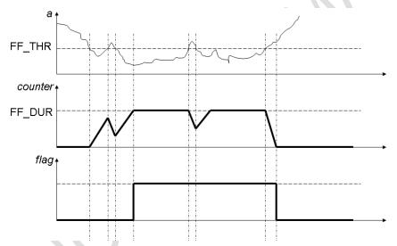
The figure above shows a simplified example with just one axis. An example acceleration input signal (simplified to only show one axis), qualifying sample counter, and Free Fall flag are shown.
