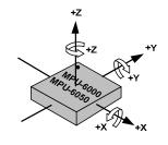
QFN Package 24-pin, 4mm x 4mm x 0.9mm QFN Package 24-pin, 4mm x 4mm x 0.9mm Orientation of Axes of Sensitivity and Polarity of Rotation
