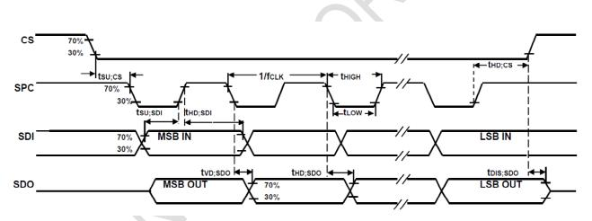
**SPI Bus Timing Diagram**
